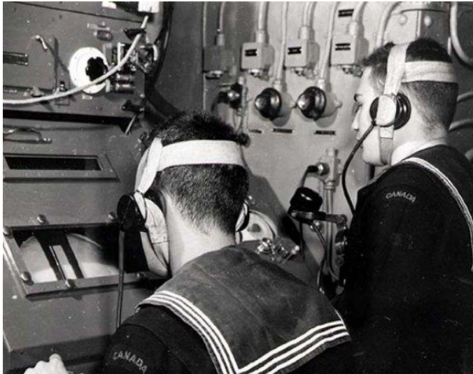
Naval Gunnery Radar. Used for targeting enemy ships.
