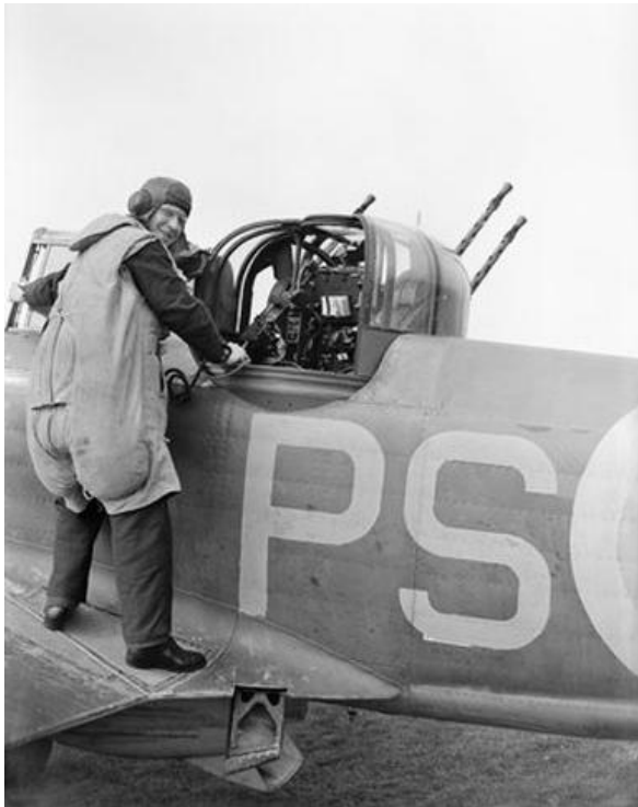
Defiant Gunner in GQ Parasuit, specially developed for use in the cramped turret.
