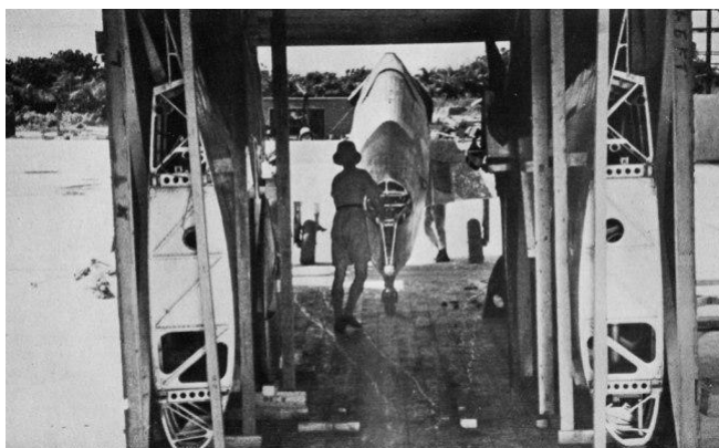
One RAF aircraft is seen being un-crated at Takoradi. The aircraft would be assembled and then start out on its perilous journey. Roughly 6,000 aircraft flew across the desert to Cairo, their final destination.
